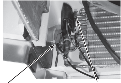
Pipe temperature/liquid thermistor (TH2)
